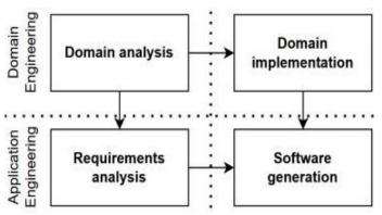
Fig. 1. Phases of software product line engineering.
